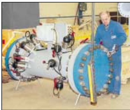
Dry calibration of Q.Sonic ultrasonic gas meter
